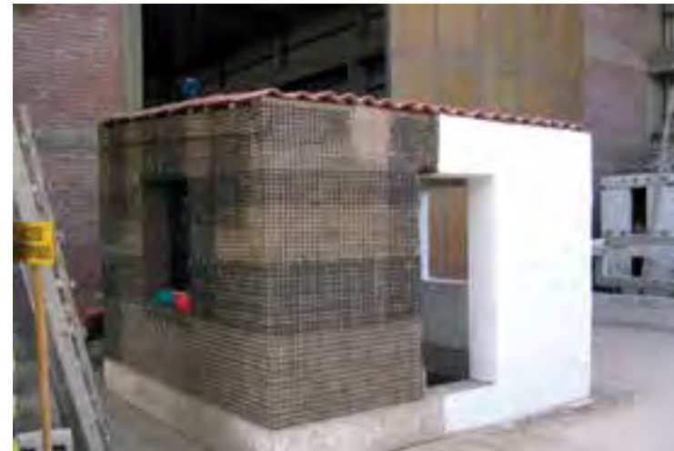
Fig.4 Module reinforced with synthetic mesh or geogrid with total reinforcement and coating of half of the module (credits: File PUCP, 2007)
