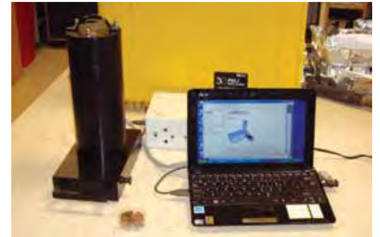
Fig.5 Portable luminescence-measurement apparatus comprising sample chamber with attached photomultiplier, control box, and laptop PC; sample in foreground (credits: Paul Adderley, 2012)
