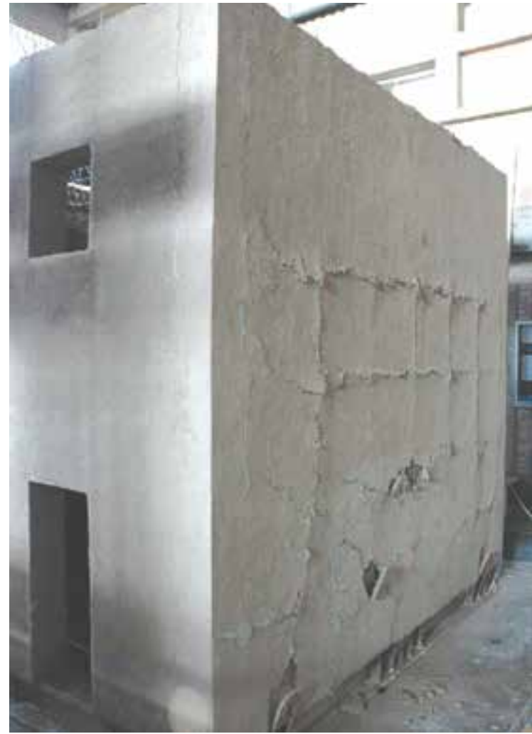
Fig.5 Detachments and cracks of the geogrid-reinforced plaster coating on the side perpendicular to the direction of the earthquake-movement simulation, after the fourth phase (displacement of 130 mm) (credits: Adell, 2008)
