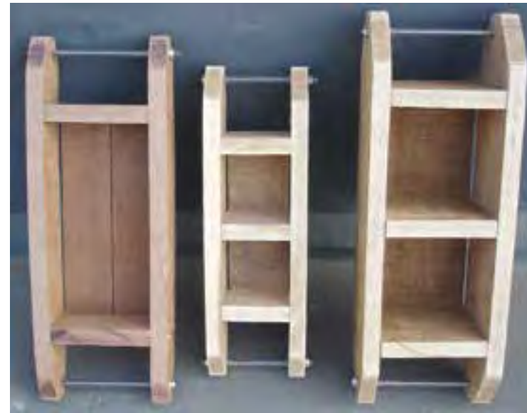
Fig.3 Molds for sample preparation (credits: Obede B. Faria, 2008)
