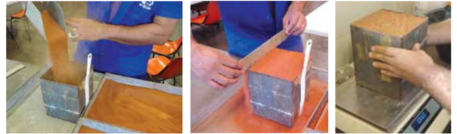
Fig.2 Determining loose soil density (credits: Obede B. Faria, 2008)
