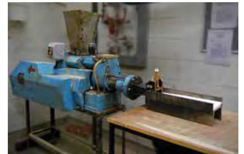
Fig.1 Laboratory vacuum pug-mill extruder (credits: Daniel Maskell)
