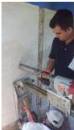
Figura 6. Ensayo de adherencia *pull-off*
