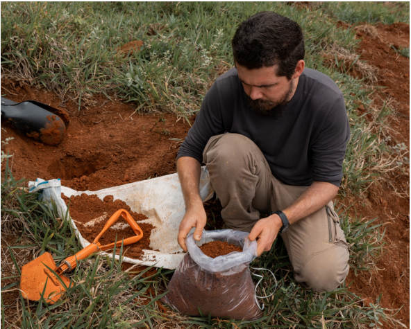
STEP 3. Store in plastic bags, tie with string, and identify the sample.
