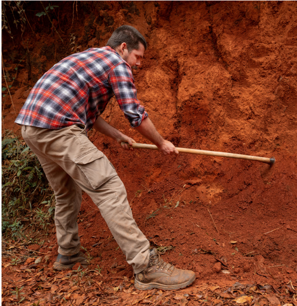
STEP 2. Remove the surface layer approximately 5 cm thick and discard.
